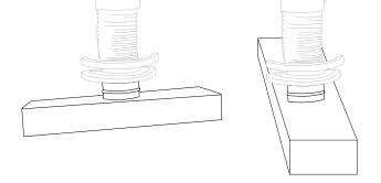
360 ° swivel function enables a wider working area and maximum flexibility
